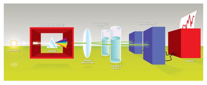
UV-visible spectrometers can be used to measure the absorbance of ultra violet or visible light by a sample, either at a single wavelength or perform a scan over a range in the spectrum. The UV region ranges from 190 to 400 nm and the visible region from 400 to 800 nm. The technique can be used both quantitatively and qualitatively. A schematic diagram of a UV-visible spectrometer is shown above.
